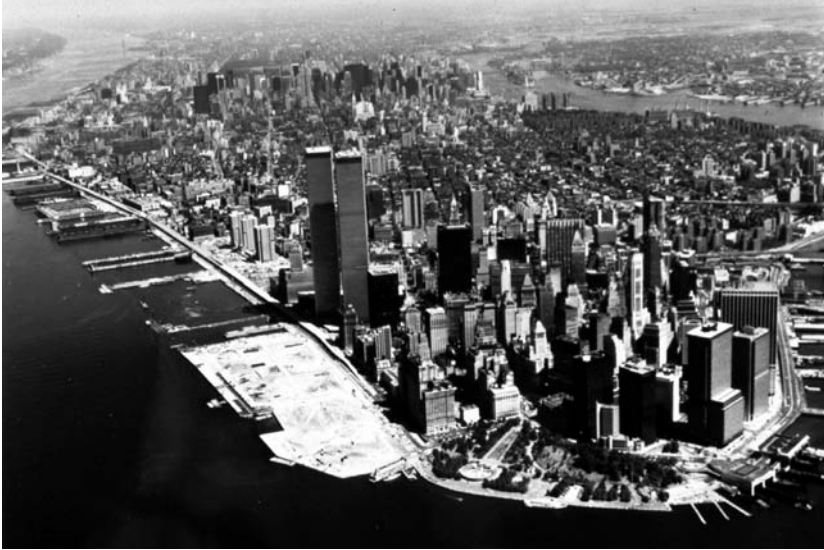
Figure 18.6. The twin towers of the World Trade Center rose 110 storeys and were visible for miles around. The landfill from the excavation (outlined in photo) would serve as the site for Battery Park City, housing more offices, housing and public amenities.
